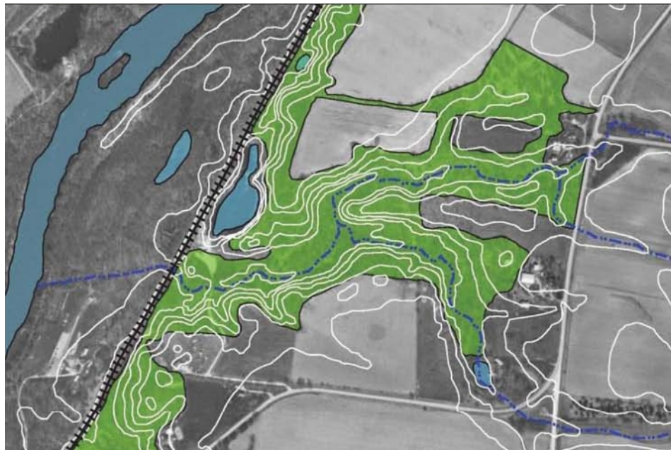
Step 2: Identifying and analyzing key environmental features such as woodlands, topography, wetlands, and natural drainage.
