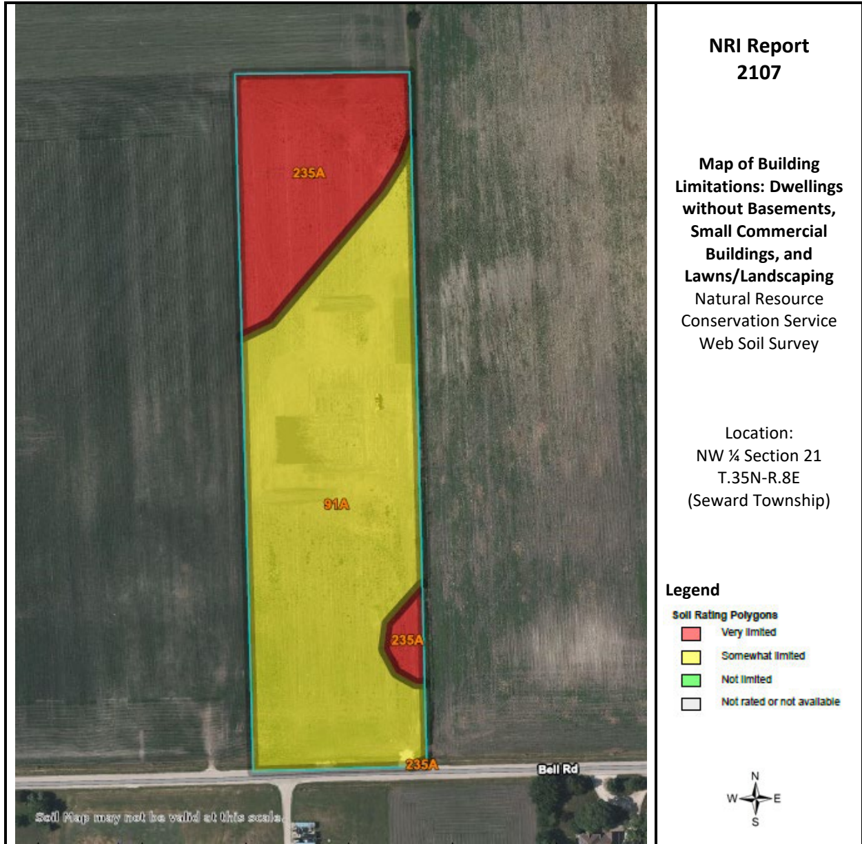
Figure 6A: Map of Building Limitations – Dwellings without Basements, Small Commercial Buildings, and Lawns/Landscaping
