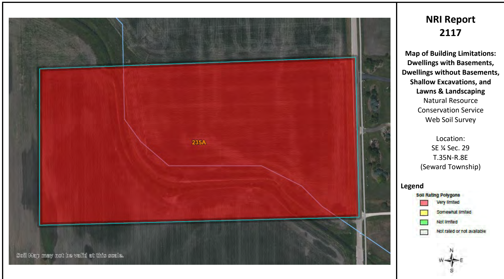
Figure 3A: Map of Building Limitations – Dwellings with Basements, Dwellings without Basements, Shallow Excavations, and Lawns & Landscaping
