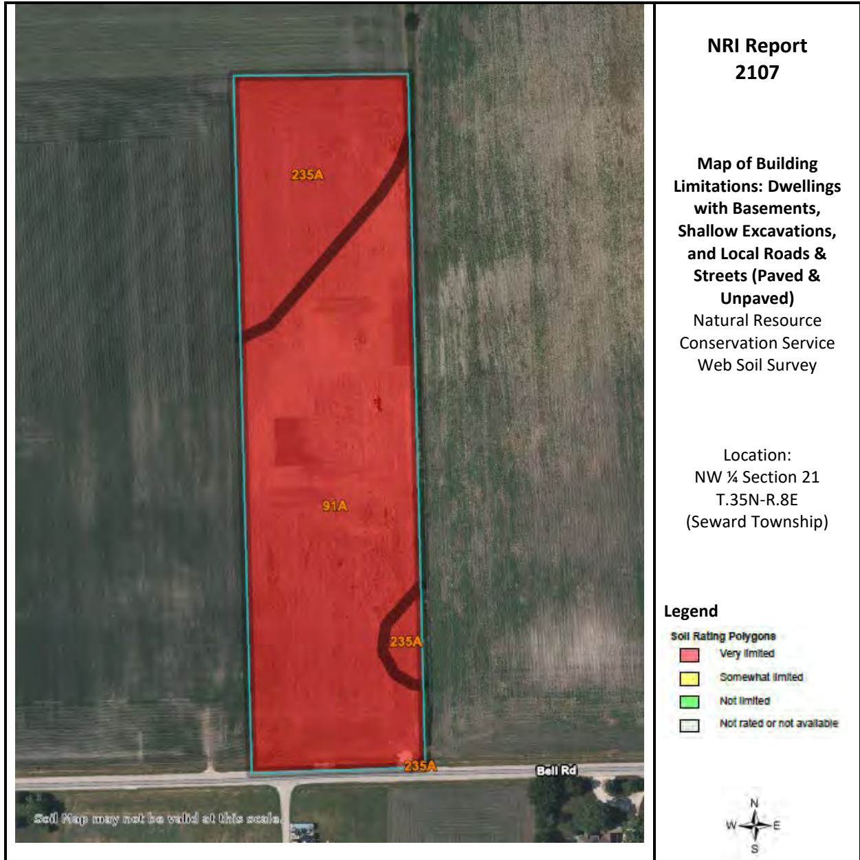
Figure 6B: Map of Building Limitations – Dwellings with Basements, Shallow Excavations, and Local Roads & Streets (Paved & Unpaved)
