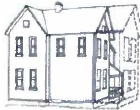
Inappropriate: Side Two-Story Addition
