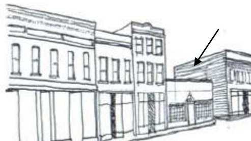
Inappropriate commercial infill
