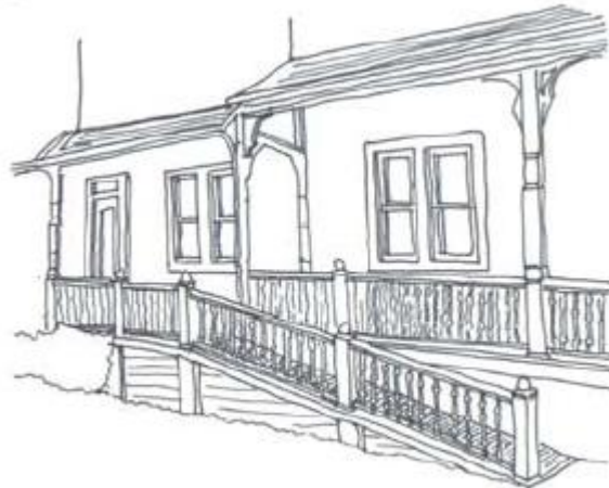
Ramp Addition to a porch
