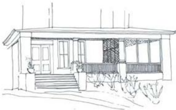
Appropriate porch screening - screens do not obstruct architectural features
