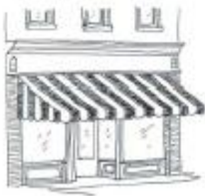
Awnings should reinforce openings, not cover features
