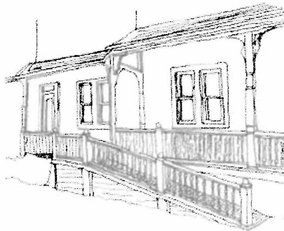
Ramp Addition to a porch
