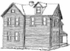
Dormer addition on rear roof
