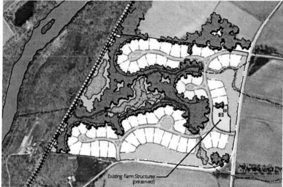
Step 4: Preparing a site design with residential lots, a road network, and conservation areas.
